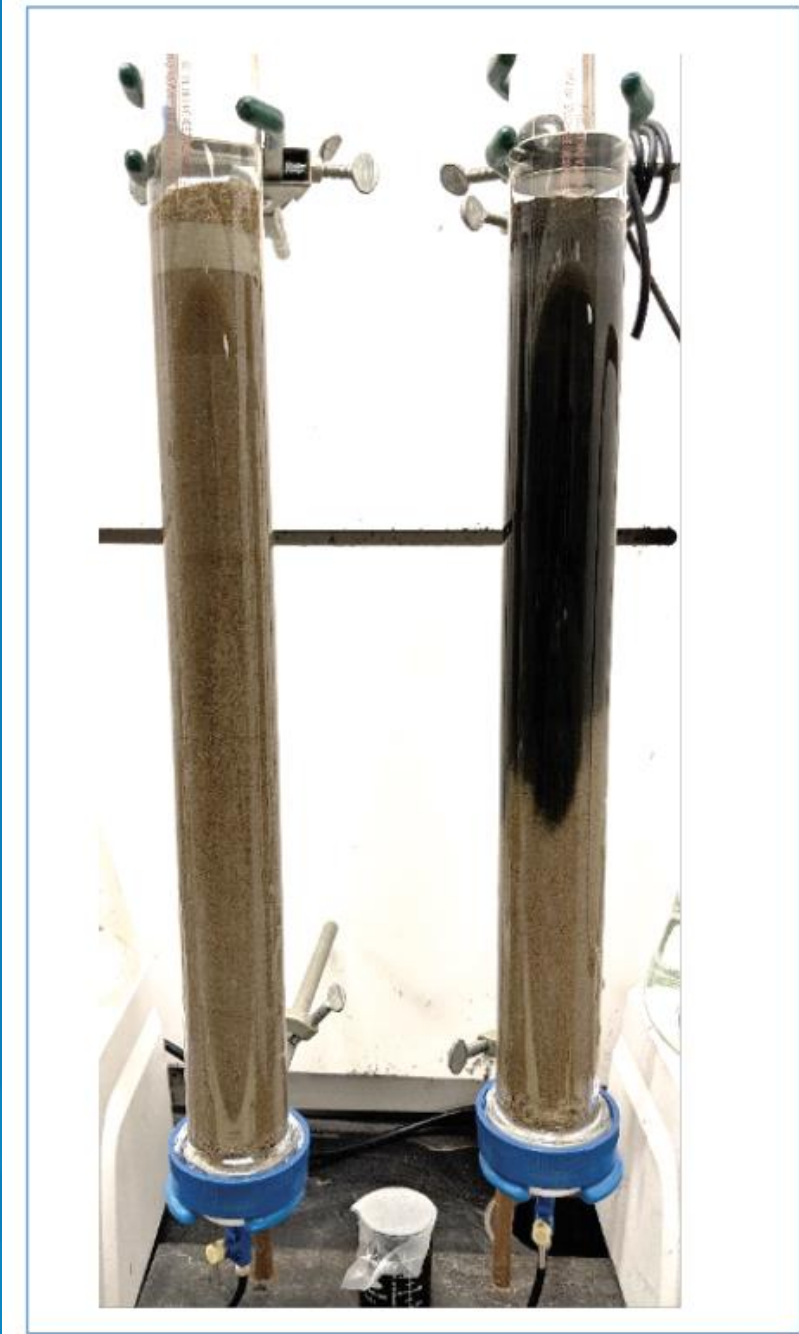
Fig 6. The control (left) and PetroFix-treated (right) columns used in the study to demonstrate the ability of PetroFix to capture small diesel spills.
