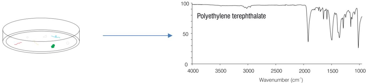
Chemical characterisation of MPs is most commonly achieved through IR spectroscopy: FT-IR and Raman.
